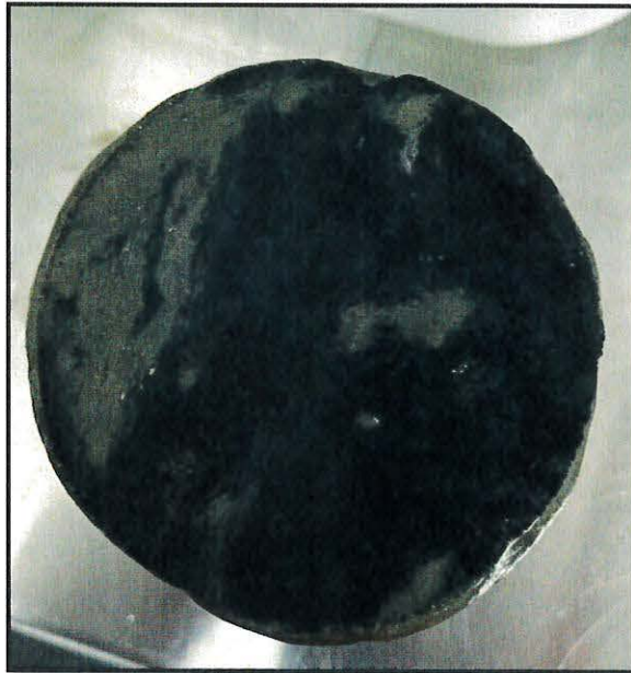
PHOTOGRAPH #1: Sample ST1 after completion of hydraulic conductivity testing.
