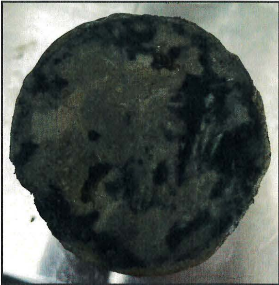
PHOTOGRAPH #1: Sample ST1 after completion of hydraulic conductivity testing.
